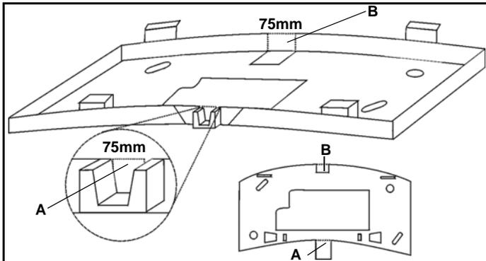
Use a knife to cut away two squares approx. 75mm from the Annunciator's back plate. Cut a square in front of the guide clip (space A) and at the top of the rim (space B). Dotted lines indicate cutting lines.
